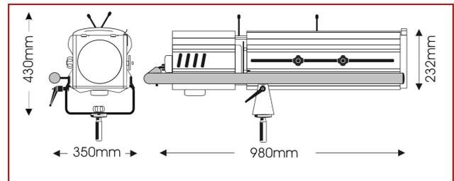
The most powerful dimmable tungsten halogen followspot in the Canto® range, the 2000W has been completely re-engineered to offer the market an even wider and better set of features. A large, user-friendly side handle, new mechanics on the mechanical dimmer and a number of "invisible" new features add to the existing specifications which have made Canto® a world-wide success.
